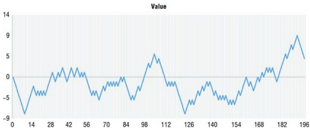
Figure 4.5 A stochastic model of tossing a coin and moving according to the results.
